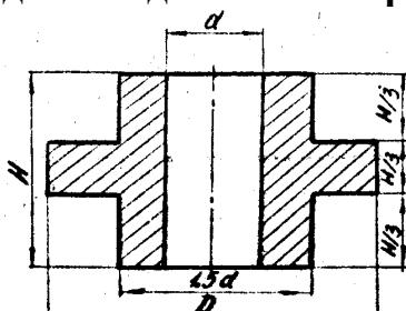
$$\begin{aligned}D &= 70 \text{ мм;} \\d &= 30 \text{ мм;} \\H &= 30 \text{ мм.}\end{aligned}$$
